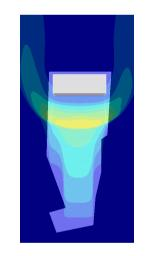
The wind is dammed up by the building. It makes the stagnant period of the wind in the area. The building location is planned to enhance the effect of the air purification.
