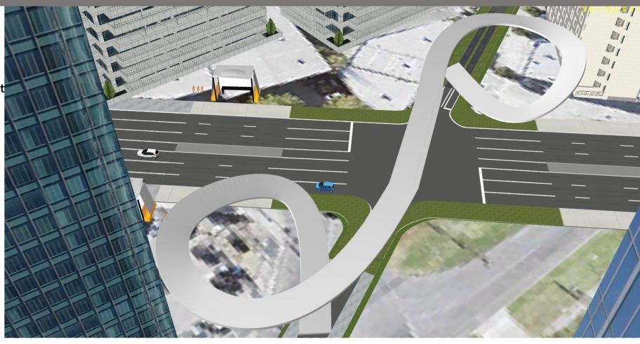
A bicycle overpass has been placed as shown to connect a divided section within the precinct. This was considered the safest means of bicycle travel through the intersection. Further separation between vehicles and bicycles
