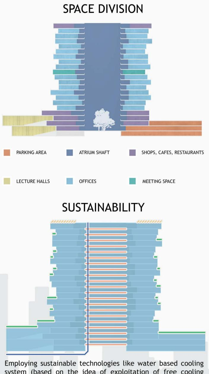
Employing sustainable technologies like water based cooling system (based on the idea of exploitation of free cooling resources from the river), green energy floor tiles (which convert kinetic energy into electricity through electromagnetic induction) and solar panels Shifting Towers strives to limit its carbon dioxide footprint and create a healthier environment for inhabitants of Shanghai.
