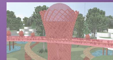
The platform and corridor become the refuge platform while water disaster coming. There are four escape ladders on each platform. This test explores the evacuation capacity of each platform.
