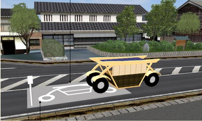
Charge system : It can be recharged simply by parking in a specific parking lot.
